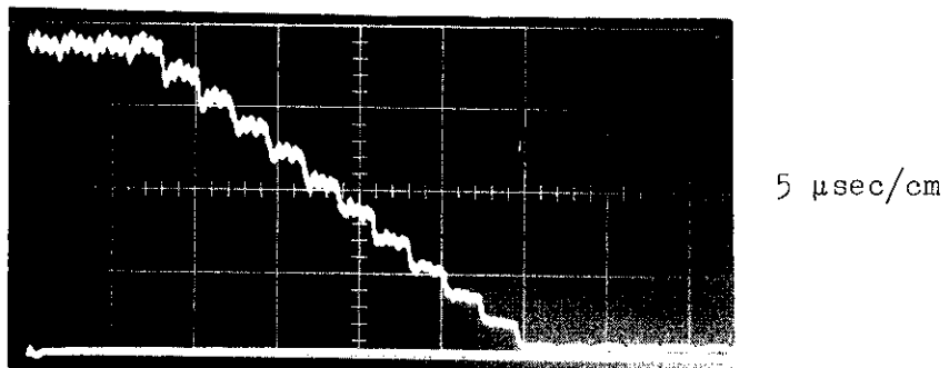
Fig. 12 Falling intensity of PS circulating beam over 11 turns corresponding to ejected beam intensity of Fig. 11
